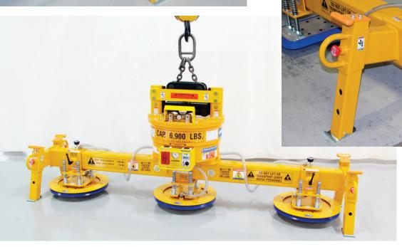
Spring loaded red knob will snap into position and lock the parking stands as you adjust them. The pin diameter is a robust one inch (25.4 mm) for security even on heavy lifters. Slanted "A" Frame construction ensures stablility.
