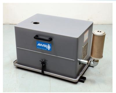
ANVER sound deadening enclosures are built from durable, melt-resistant, industrial-quality plastic. They have a steel base plate and are fully lined with sound deadening material. Service temperature rating: -40°F (-40°C) to +225°F (+107°C) continuous to +275°F (+135°C) intermittent. ANVER recommends purchasing the enclosures with the vacuum station as they require special plumbing. Note, when ordering sound enclosures at a later date, additional fittings are required.
