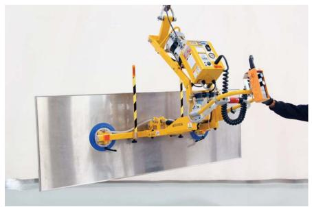
ANVER's Upender 180° Flipper is a C-frame style lifter that lets one person lift sheets and panels, invert them, inspect the other side, and then place them in jigs for assembly or secondary operations. Featuring two double vacuum suction pads to assure even loading and stress-free handling.
