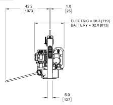
NOTE: Maximum lifter capacity and lifter weight combined can not exceed 22,500 LB (10,205 KG).
