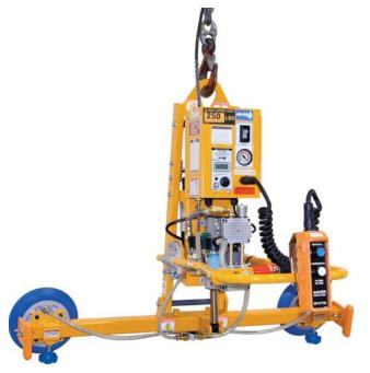
Anver Vacuum Tilters and Upenders are loaded with safety features and have come to set the standard for safe tilting of loads. Each version has been revised over the years to perform better and last longer. The pads, vacuum generators, frame, controls, hardware, filters, safety features and handlebars etc are all new and improved. Every aspect of the lifters has been redesigned and the latest represent the best Tilters available.
