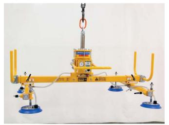
ANVER'S Standard Vacuum Lifters offer efficient material handling solutions by promoting functionality, safety, and ergonomic operations for a wide variety of applications and materials. Standard lifting frames are built to order from stock using modular components, so there are hundreds of possible combinations depending on the vacuum generator, beam, crossarms, and vacuum cups selected.
