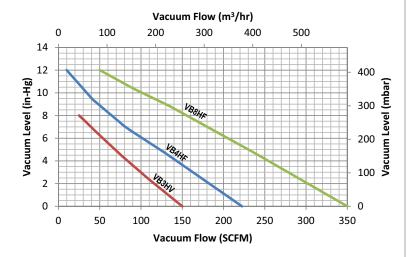
High Flow Pumps are especially suitable for porous load applications. They produce air flows up to 350 SCFM making them a natural choice for lifting porous and semi-porous loads. The three pump models available with varying capacities are listed in the High Flow Pump Specifications table below.
