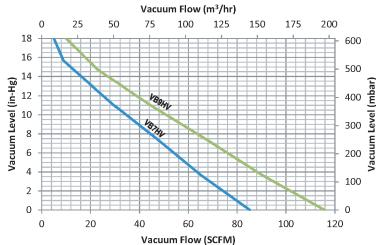
High-Vacuum Pumps produce vacuum up to 18 in. Hg, which makes them an ideal choice to lift heavy, non-porous to semi-porous loads. The two pump models available with varying capacities are listed in the High Vacuum Pump Specifications table below.
