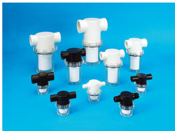
ANVER vacuum filters range in size from 1/4" to 1-1/2" NPT and are constructed from FDA approved black nylon. If space permits, use of the longer size bowl will require fewer element changes. These are for use with vacuum pumps and vacuum systems. They are 100% airtight, even after repeated element changes; you can easily see when the element needs changing; they do not corrode or rust; and the element works well even on fine dust.
