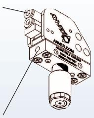
Threaded Vacuum Ports on both ends, (fits M5 or 10-32 thread), allows for series connection, or insert plug in one end for single vacuum line connection. Supplied with one threaded plug, part no. SPG-10.
