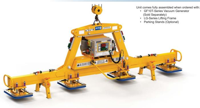
ANVER'S standard lifting frames are built to order using modular components, so there are hundreds of possible combinations depending on the vacuum generator, beam, crossarms and vacuum cups selected.
