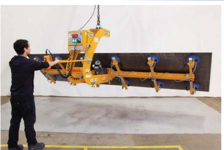
ANVER's Upender 180° Flipper is a C-frame style lifter that lets one person lift sheets and panels, invert them, inspect the other side, and then place them in jigs for assembly or secondary operations. Featuring twelve vacuum suction pads to assure even loading and stress-free handling.
