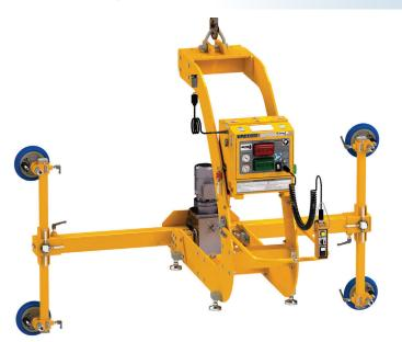
ANVER's Upender 180° Flipper is a C-frame style lifter that lets one person lift sheets and panels, invert them, inspect the other side, and then place them in jigs for assembly or secondary operations. Featuring four vacuum suction pads to assure even loading and stress-free handling.
