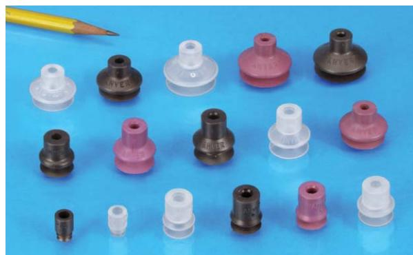
1.5 Bellows Vacuum Suction Cups attach gently and easily with minimum pressure. Excellent for most concave and convex shapes, bellows suction cups attach to curvatures such as containers, bottles, cylinders, etc., and can be used in any orientation. Their spring action compensates for height variances in the load or machine inaccuracies. The bellows suction cup design duplicates the function of mechanical springs and ball-joint connectors in a much smaller and more economical package.
