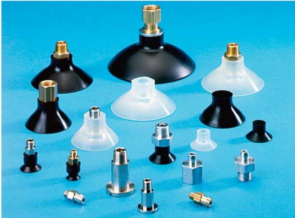
Flat vacuum suction cups attach quickly due to the small volume of air to be evacuated. They feature patterned knobs on the bottom to maximize capacity and are excellent for holding flat, flexible materials without deformation. Relatively stiff, the cup bodies retain their shape well in production applications. They are excellent for use on fast cycle transfer systems. Use on flat or slightly curved surfaces, and for horizontal or vertical lifting.
