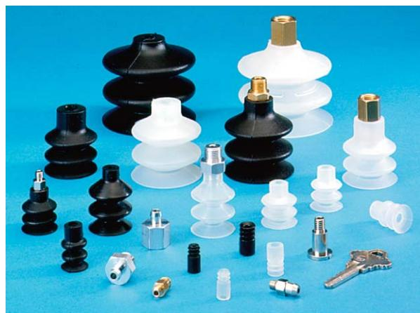
2.5 Bellows Vacuum Suction Cups attach gently and easily with minimum pressure. They are excellent for concave and convex shapes as well as on slanted surfaces. Their design can replace mechanical springs, ball swivels and height compensators, allowing for less complicated and more economical installations. Keeping vacuum levels a bit lower extends the life of the suction cups.
