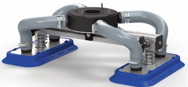
T-Series pads attach to aluminum beam for adjustable width. Dual NPT ports allow for maximum airflow. Beam assembly can be paired with quick release for highest efficiency.
